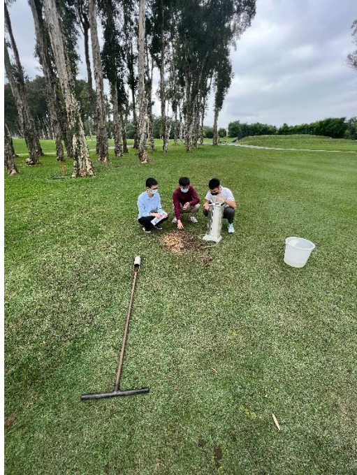
Figure 6. HKU team conducting K-sat experiment at Fanling golf course site.
