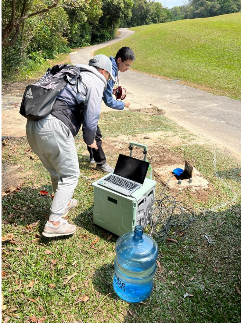
Figure 8. HKU team conducting Falling-head test at the Fanling golf course sites
